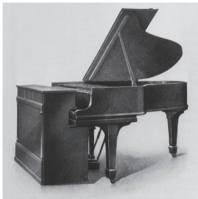
Photo 1: Welte Mignon "Vorsetzer" in position at the piano
